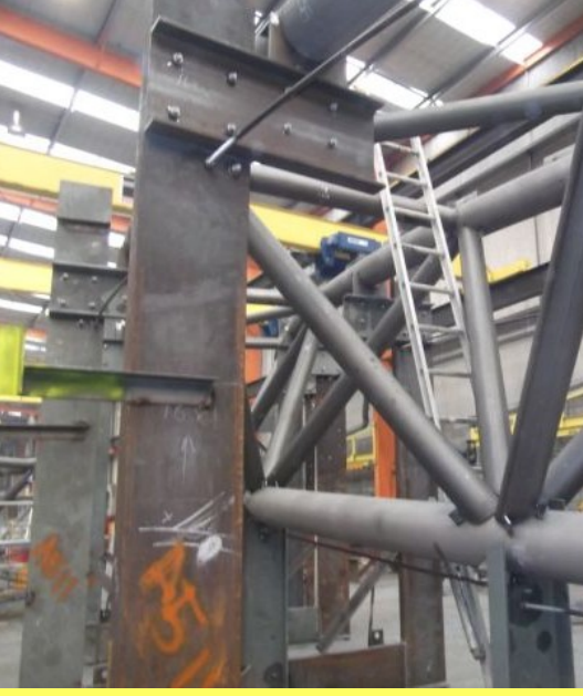
The 10-tonne jig on which each tubular truss is precisely formed.
